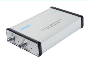
Combine DTU-238 with *RFXpert* software for RF measurements and with *StreamXpert* for real-time Transport-Stream analysis
